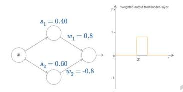
To simplify notation, we can introduce parameter h for the height (instead than  $w_1$  and  $w_2 = -w_1$ ).
