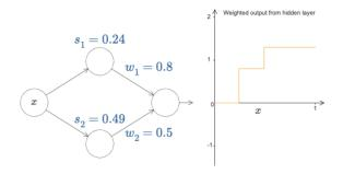
The plot is for  $w_1a_1 + w_2a_2$  where  $a_1$  and  $a_2$  are the *activations* of the top and bottom hidden neurons. This is different from the output of the net, which computes  $\sigma(w_1a_1 + w_2a_2 + b)$  where b is the bias of the output neuron.
